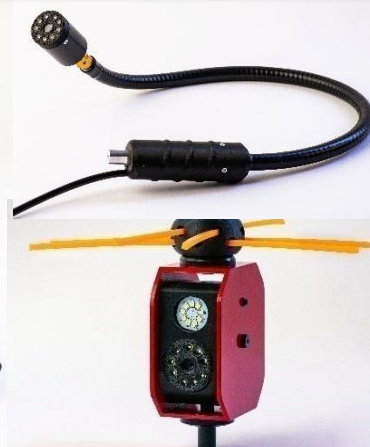
ENVIRO CAMERA WITH GOOSENECK (ABOVE) AND ENVIRO IN CHEESEBIT
