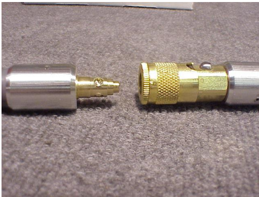
1) Simply align male end into connector
