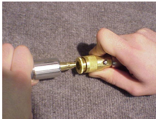
2) Pull back the indented ring past the button. Push the male into the connector. Roll the male end till the ring will release.
